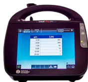
Lasair® III Pro Airborne Particle Counter Sensitivity range: 0.3 - 25.0 \mu\text{m}
